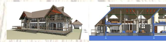
Some illustrations of how the design of thatched roof structures can be done using the latest technology – the colour coding identify different structural members.
