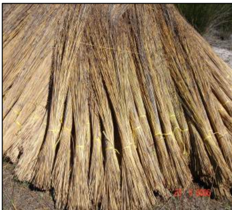
Good quality Cape reed stacked correctly
