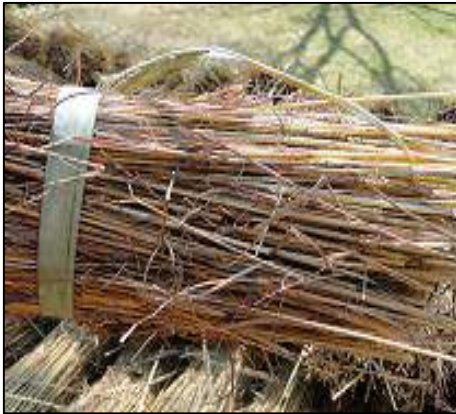
Poor thatch uncombed at harvesting contains loose material
