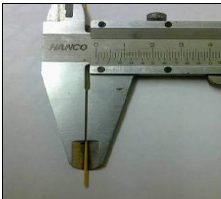
Incorrect diameter of butt end: 1mm.
