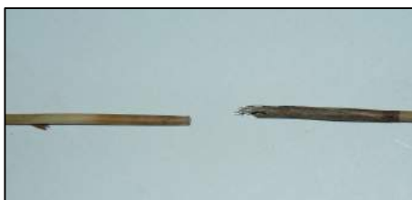
This slide shows that this reed has been cut in the growing season (therefore the nodes are loose)
