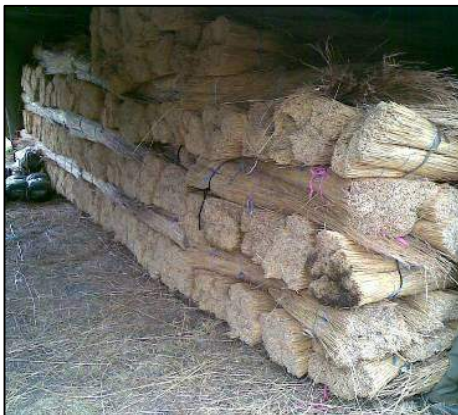
Correct storage of thatch grass on site
