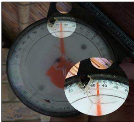
Correct Primary Roof Pitch @ 45° or more
