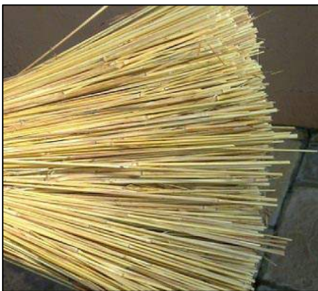
Properly harvested thatch free of any loose material
