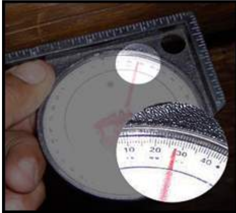
Incorrect Roof Pitch @ less than the required 45°
