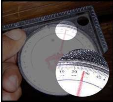
Incorrect Roof Pitch @ less than the required 45°
