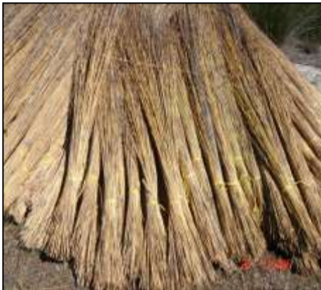
Good quality Cape reed stacked correctly
