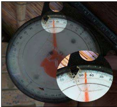
Correct Primary Roof Pitch @ 45° or more
