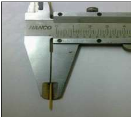
Incorrect diameter of butt end: 1mm.
