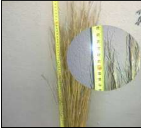
Incorrect cut length of 0.75m
