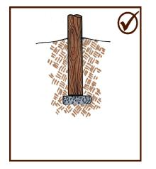
If you plant the post on concrete at the bottom of the hole, let the concrete set before planting the post.
