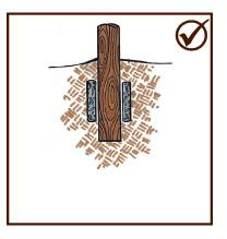
If you need to use concrete then let the concrete form a collar around the post with the end of the post protruding through the concrete.
