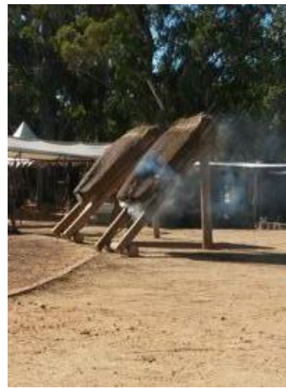
Demonstration of the performance of a chemical fire retardant product
