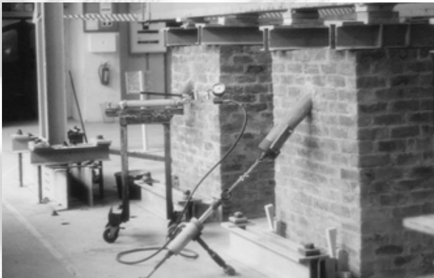
Photograph 14 Experimental test set-up to determine rafter pull- out force from walls
