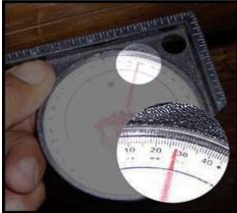
Incorrect Roof Pitch @ less than the required 45°
