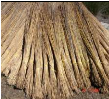
Good quality Cape reed stacked correctly
