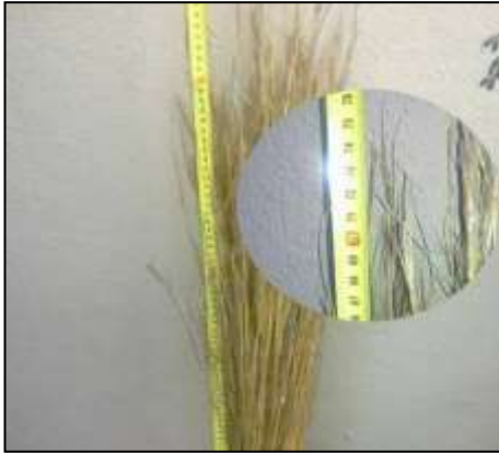
Incorrect cut length of 0.75m
