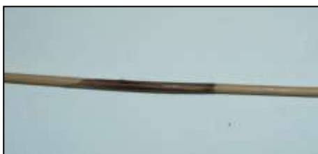
Intact nodes cut out of the growing season (Therefore nodes are tight)
