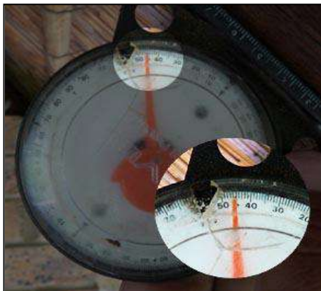
Correct Primary Roof Pitch @ 45° or more
