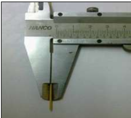
Incorrect diameter of butt end: 1mm.
